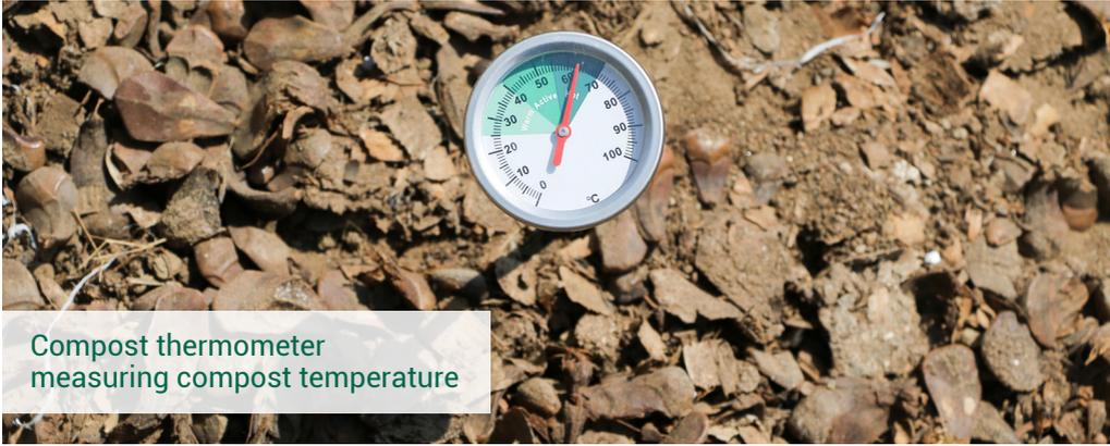
Compost thermometer measuring compost temperature
